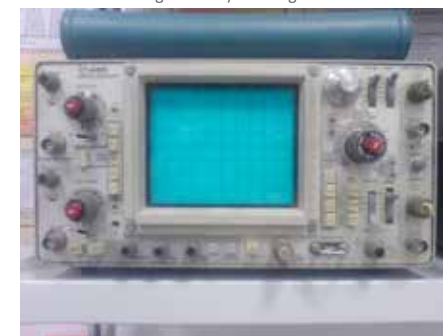
Figure 3: Dual-channel oscilloscope to measure the time delays
