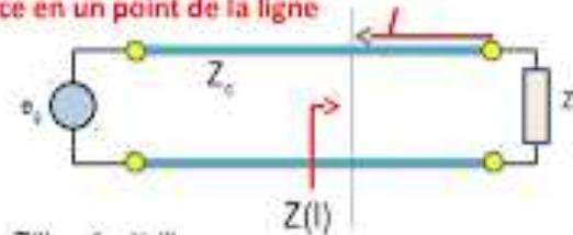
$$z(l) = \frac{Z(l)}{Z_c} = \frac{1 + \Gamma_c(l)}{1 - \Gamma_c(l)}$$
